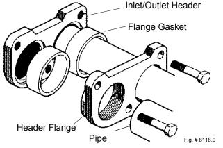
**CAUTION:** Never install PVC directly in header flanges. The initial connection must be made with a higher temperature material such as CPVC or Copper. PVC may be utilized immediately after the initial connection.
